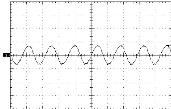
Figure 8. Input Reflected Ripple Current (10mA/div) time scale - 2µS/div. Vin=Vin\_nom, full resistive.
