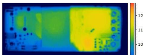
Thermal Image of module @ 48Vin, 200LFM & 70C
