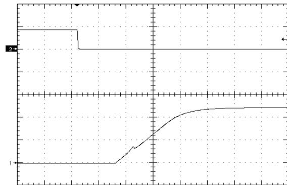
Figure 10. Startup Waveform via Enable Pin, time scale 4ms/div. Vin=Vin\_nom, full load + 10000µF (neg. enable.) Ch1=2V/div,Ch2=5V/div
