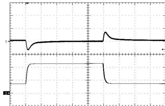
Figure 12. Load Transient Response (100mV/div), di/dt=0.1A/µS, 25% - 75% - 25% of full load, +4700µF, time scale: 200µS/div
