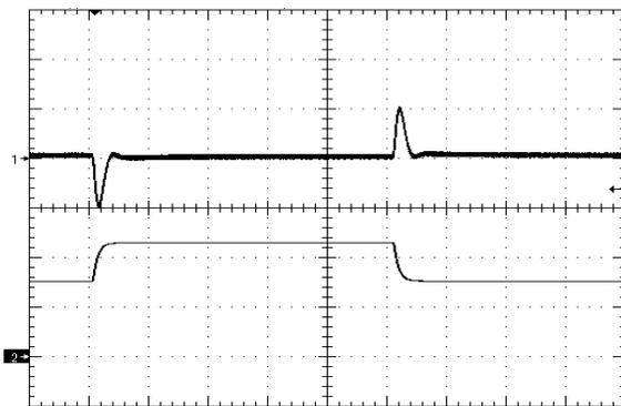
Figure 11. Load Transient Response (100mV/div), di/dt=0.1A/µS, 50% - 75% - 50% of full load, time scale: 200µS/div.
