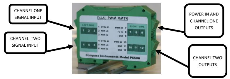
The Compass Instruments P550A Dual PWM Transmitter is a dual voltage to pulse width modulator.
