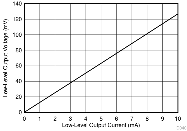
Figure 6-37. Low-Level Output Voltage vs. Low-Level Output Current
