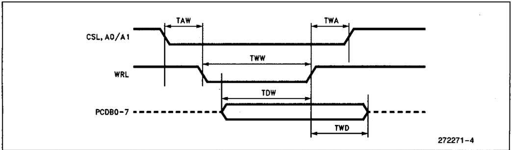
Figure 4. Host-Interface Write
