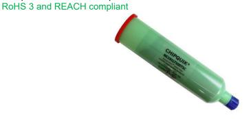
\*Shelf Life Notes: Chip Quik® solder paste is good past its quoted shelf life, regardless of refrigeration. Before use, visually inspect the solder paste to ensure it is not dried out or clumpy, or check stencil release. If stored in a jar, stir the product thoroughly for 2-3 minutes before inspection and use.
