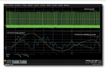
Information on the steering angle and steering angle rate of change is extracted from the CAN message acquisition, rescaled to decimal values, and plotted as a time-correlated "Track"
