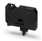
Fuse plug, Prior to replacing the cartridge fuse, disconnect the fuse connector from the basic terminal block., nominal current: 10 A, connection method: Plug-in connection, fuse type: G / 6,3 x 32, mounting type: Plug-in mounting, color: black
