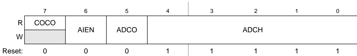
Figure 10-3. Status and Control Register (ADCSC1)
