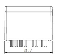
Note :1.The dimensional tolerance without directions is  $\pm$  0.5mm.
