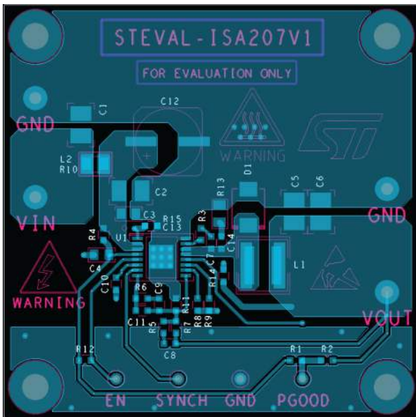
Figure 16. Demonstration board layout (top)
