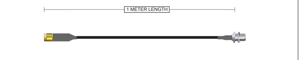
Connector A 132451 SMA Plug Straight Brass Gold + Heatshrink 50 Ohm LMR-240 Continuity/Hi-Pot
