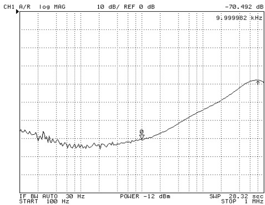
Figure 12. LDO3/4 PSRR vs. Frequency, 50 mA Load
