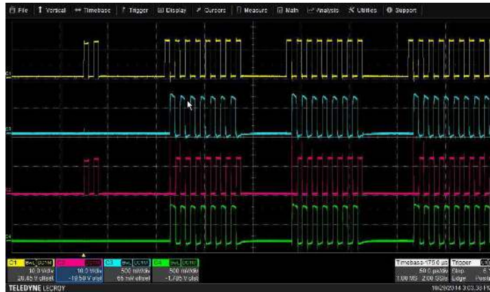
Figure 27. UCC28950 Burst-Mode Function
