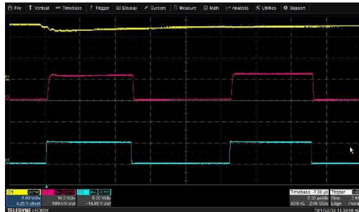
Figure 22. VDD Drop On First Bootstrap Capacitor Charging
