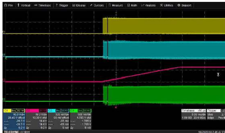
Figure 28. UCC28950 Burst-Mode Function During Soft Start
