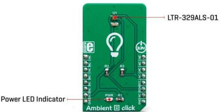
The LTR-329ALS-01 sensor uses a set of configuration registers, which allow very simple operation. By default, the ALS sensor is set to the standby mode. It does not perform any conversions until set up in the active mode. The Click board<sup>™</sup> is supported by the mikroSDK compatible library, which simplifies the development by offering simple functions. However, more detailed explanation of each register and its function can be found in the datasheet of the LTR-329ALS-01.
