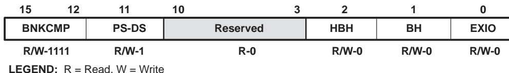
Figure 6. Bank-Switching Control Register (BSCR), MMR Address 0029h
