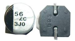
Rated for 125°C, type HZC combines the advantages of aluminum electrolytic and aluminum polymer technology. These hybrid capacitors have the ultra-low ESR characteristics of conductive aluminum polymer capacitors packaged in a V-chip, SMT case with high capacitance and voltage ratings that were previously available only in aluminum electrolytic technology. Applications for type 125°C hybrid capacitors include a variety of industrial power conversion, lighting control and automotive applications.
