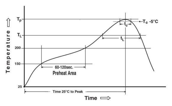
Preheating temperature:  $150 \sim 200$ °C,  $60 \sim 120$  seconds Liquidus temperature (TL): 217°C,  $60 \sim 150$  seconds
