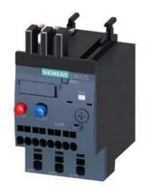
Overload relay 7.0...10 A Thermal For motor protection Size S00, Class 10 Contactor mounting Main circuit: Spring-type terminal Auxiliary circuit: spring-type terminal Manual-Automatic-Reset
