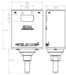
\*Dimensions are drawn with 1/8" NPT fitting installed
