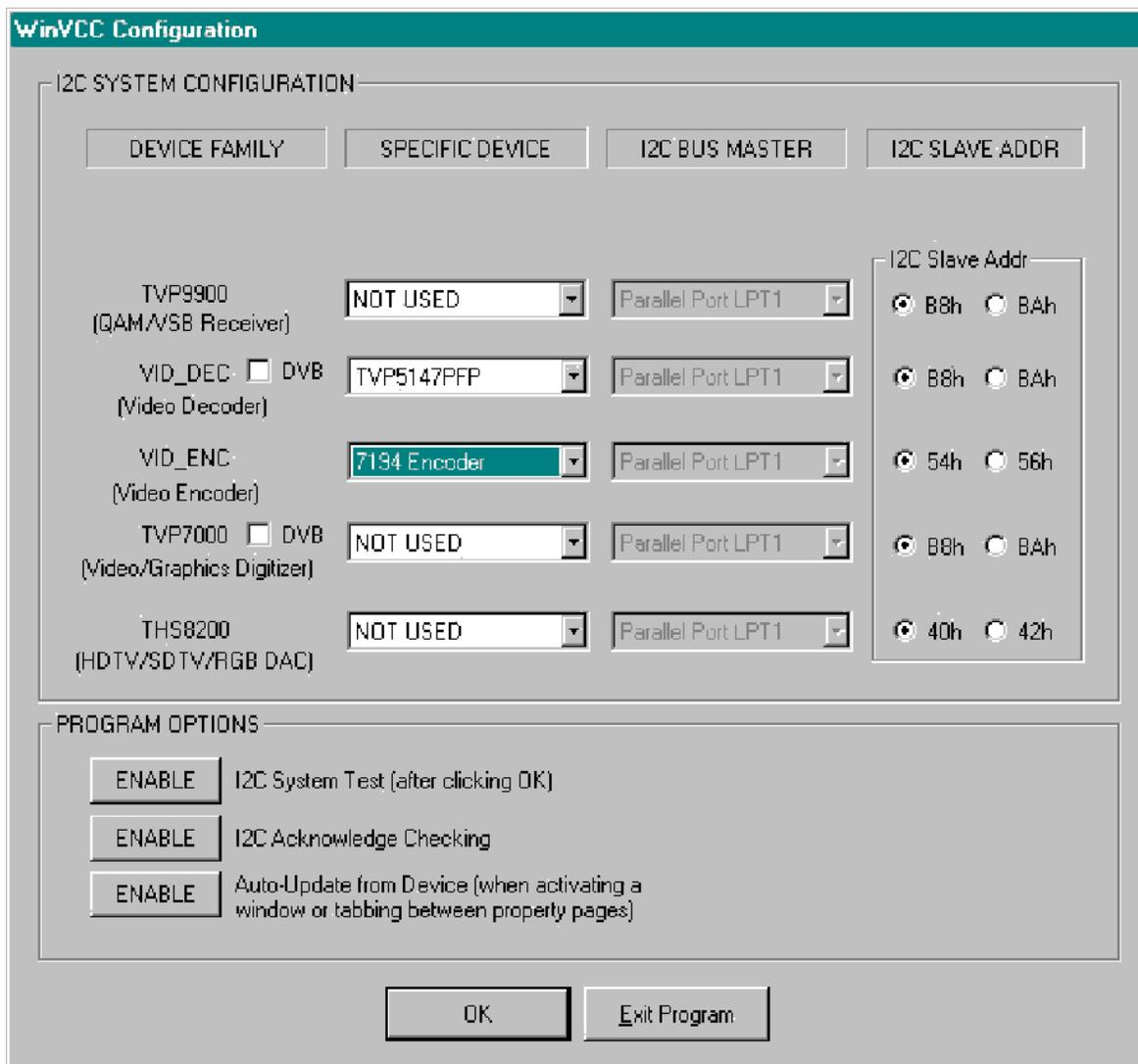
**Figure 3-1. WinVCC I<sup>2</sup>C Address Configuration**
