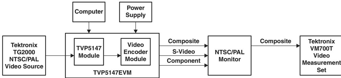
**Figure 1-5. TVP5147EVM System Level Block Diagram**
