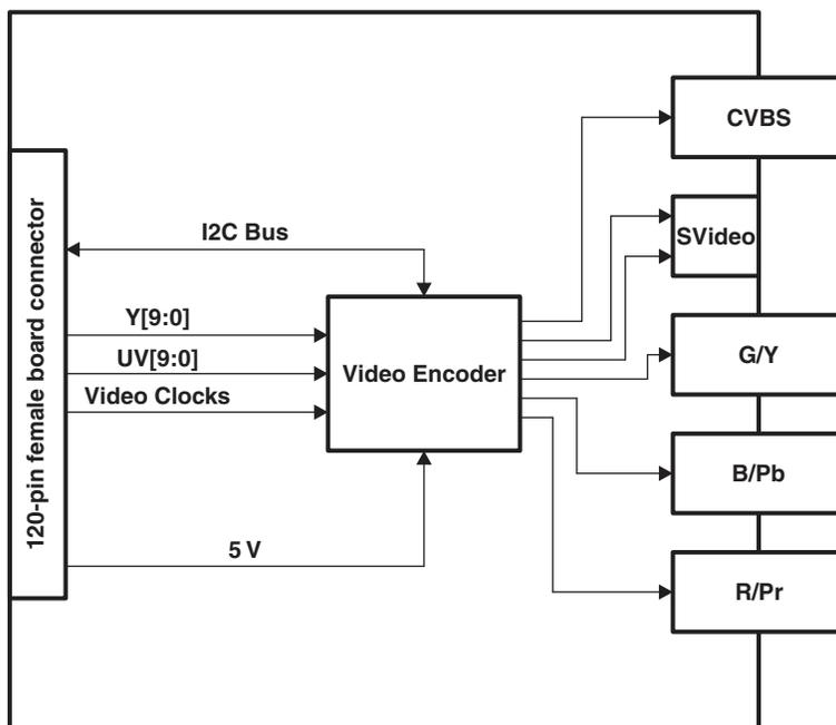
Figure 1-2. Encoder Module
