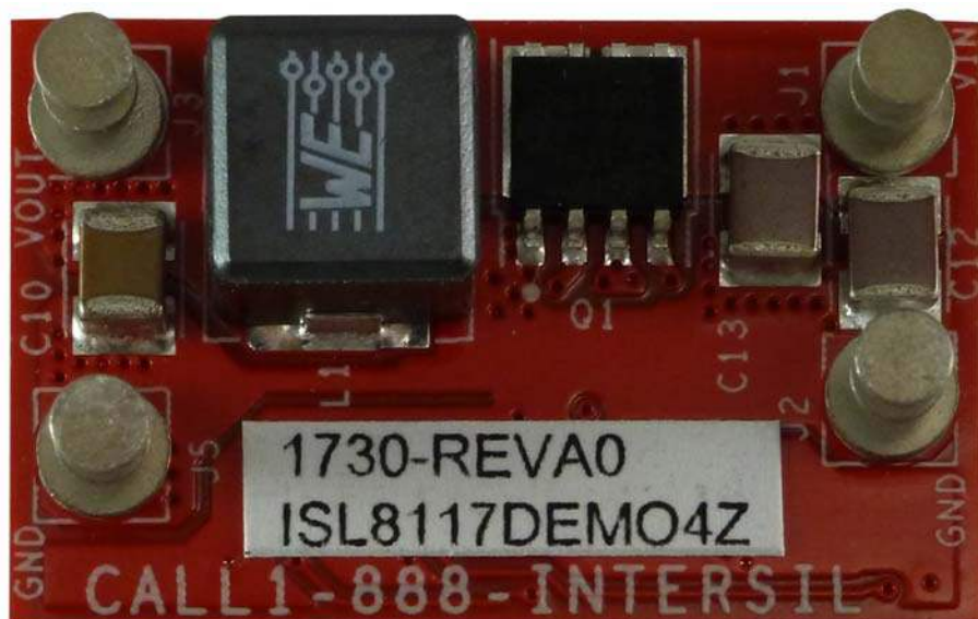
Figure 5. ISL8117DEMO4Z Bottom Side
