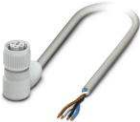
Sensor/Actuator cable, 4-position, PP-EPDM halogen-free, Gray RAL 7035, Free cable end, on Socket angled M12, A-coded, with 3 LEDs, Cable length: 5 m, Hygienic design, with plastic knurl
