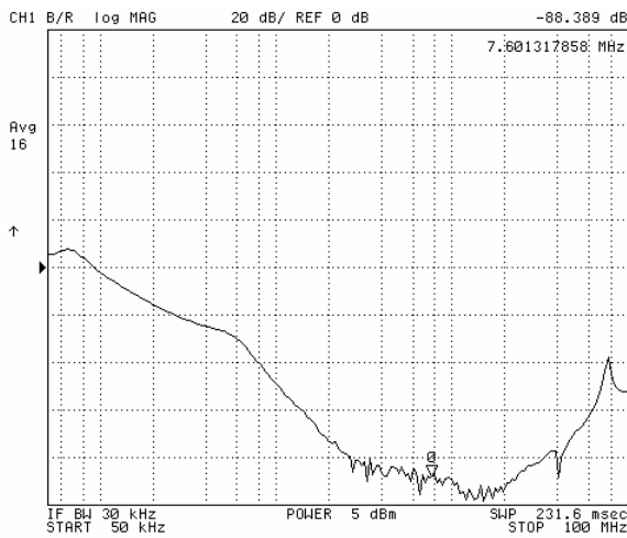
Figure 3 - Common Mode attenuation, 0.05-100 MHz. Source and load resistances are 50 Ω. Two 0.1 μF Y-caps to common line. Vertical scale: 20 dB/div, with zero dB level marked by arrow.
