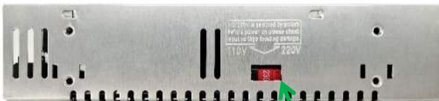
220VAC Input Voltage
