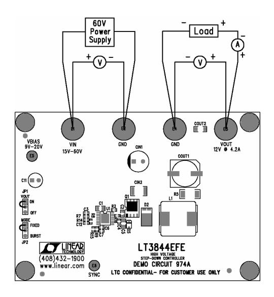
Figure 1. Proper Measurement Equipment Setup
