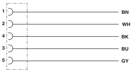
Contact assignment of the M12 socket
