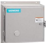
Non-reversing NEMA contactor, Size 1, Three phase full voltage, Contactor amp rating 27A, 3 wire (NO aux included), 220-240/440-480VAC 60Hz coil, Noncombination type, Encl NEMA type 4X 304 S-Steel, Water/dust tight noncorrosive, Extra-wide enclosure
