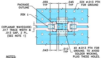
TRACE WIDTH AND GAP ARE SHOWN FOR ROGERS RO4350B WITH DIELECTRIC THICKNESS .010" ± .001".
