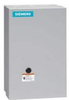
Electrically held lighting contactor, Contactor amp rating 30A, 0 N.C. / 12 N.O. Poles, 600VAC 60HZ coil, Non-combination type, (no disconnect device), Enclosure NEMA type 1, Indoor general purpose use
