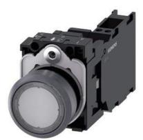
Illuminated pushbutton, 22 mm, round, plastic with metal front ring, clear, pushbutton, flat, momentary contact type, with holder, 1 NO+1 NC, LED module with integrated LED 24 V AC/DC, Spring-type terminal
