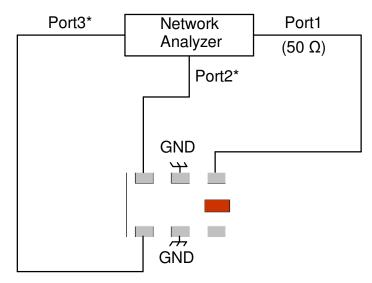
\*Impedance for ports 2 and 3=1/2(Balanced impedance)
