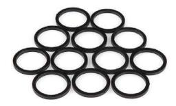
Description: These plastic shaft spacers have an inner diameter of 1/2" and a thickness of 1/16". These spacers are ideal for spacing out an area between a bearing and a shaft collar to reduce metal to metal contact.
