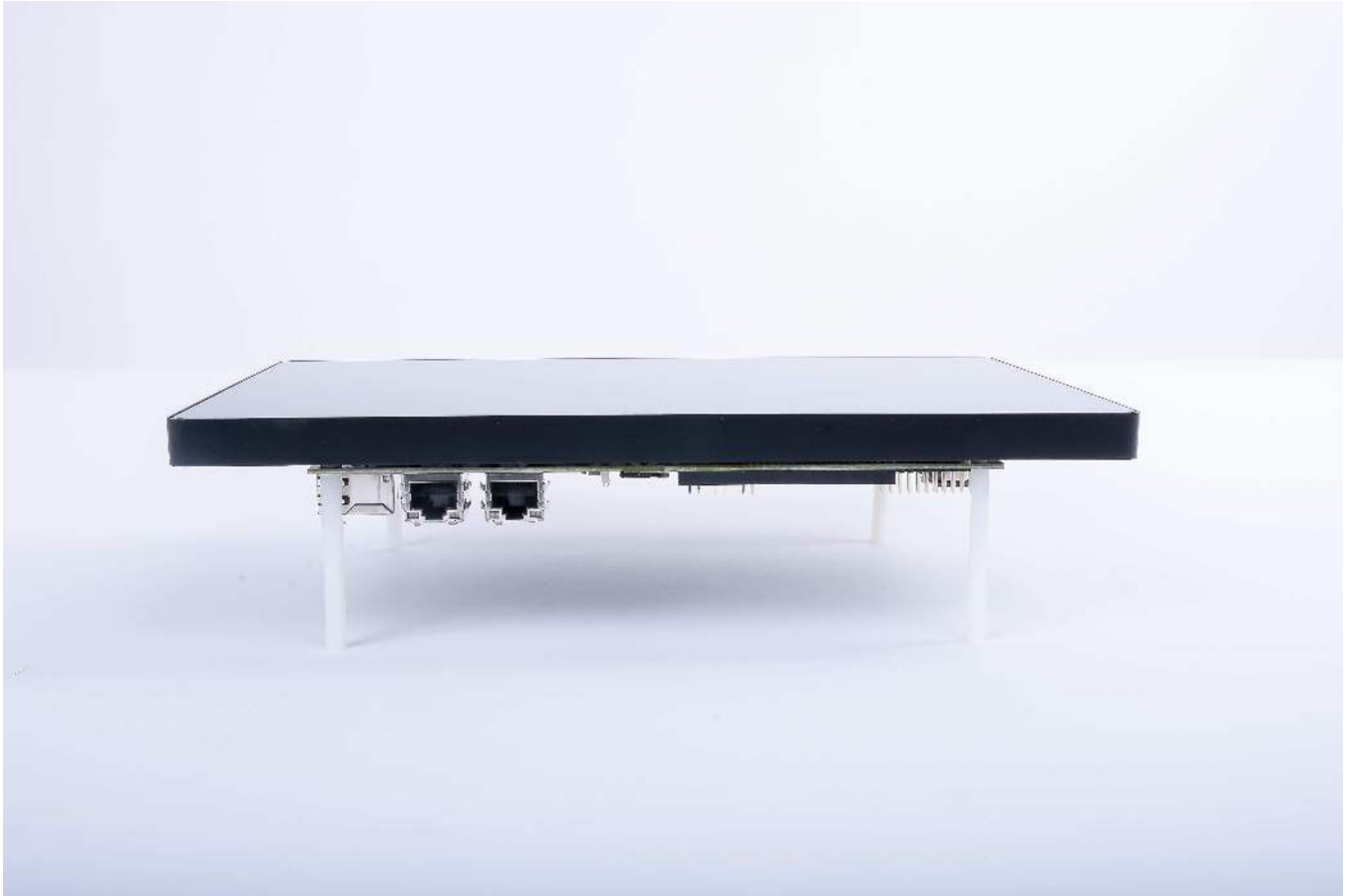
Figure 3. AM574x IDK EVM with LCD Display Assembly Attached - Top View
