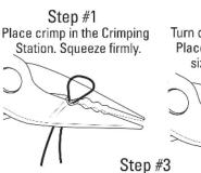
Step #2 Turn crimp on its side. < Place in the appropriate size Folding Station. Squeeze firmly.
