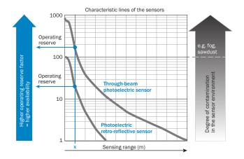
At a sensing range of "x" the photoelectric retro-reflective and through-beam photoelectric sensors have different operating reserves (see blue arrow). The higher the operating reserve factor, the better the sensor can compensate the contamination in the air or in the light beam and on the optical surfaces (front screen, reflector), i.e. the sensor has the maximum availablity, otherwise the sensor switches due to pollution although there is no object in the path of the light beam.
