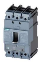
circuit breaker 3VA5 UL frame 125 breaking capacity class S 25kA @ 480 V 3-pole, line protection TM240, ATAM, In=20A overload protection Ir=16A ...20A short-circuit protection Ii=7.5...15 x In cable connection on both sides
