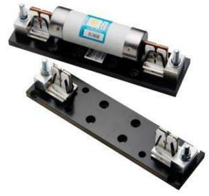
The SPFRHD series is specifically designed for 1000 Vdc SPFR fuses ranging up to 400 A in current. It is self-certified to 1000 V and UL Recognized to 600 V.
