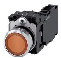
Illuminated pushbutton, 22 mm, round, metal, shiny, amber, pushbutton, flat, momentary contact type, with holder, 1 NO+1 NC, LED module with integrated LED 230 V AC, screw terminal
