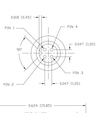
DESCRIPTION: M5 MALE - CABLE MOUNT - SOLDER CUP - 4 POSITION - SHIELDED
