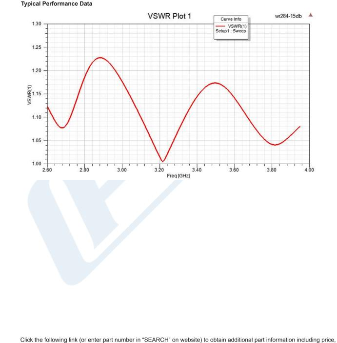
inventory and certifications: WR-284 Standard Gain Horn with 15 dBi gain, N Female connector PEWAN284-15NF
