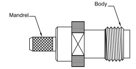
3) Insert the contact into the body and ensure that the contact captivates. Make sure that the braid is on the outside of the mandrel. Slide the ferrule over the braid until the ferrule butts up against the body. Crimp the ferrule using the correct tool for the connector.
