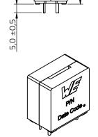
Pin 2 and 3 are only for mechanical stability.
