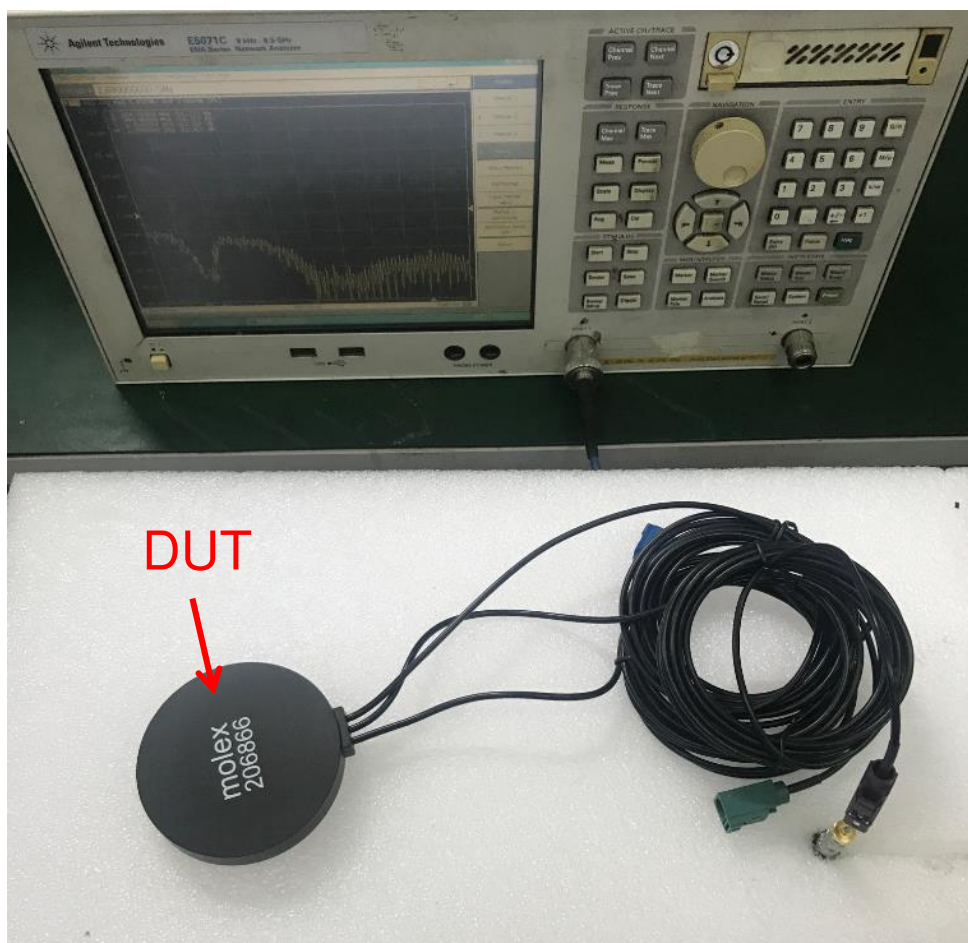
FIGURE 4.1.1 ANTENNA TESTED WITH VNA E5071C
