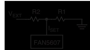
Figure 5. DC Voltage Control
