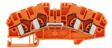
Feed-through terminal, Tension-spring connection, Mounting type: Mounting rail TS 35/7.5, Rated cross-section: 4 mm<sup>2</sup>, Width: 6.1 mm, Colour: Orange
