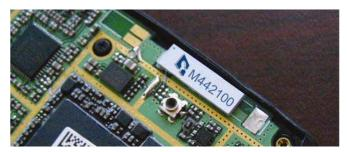
These highly innovative antennas provide competitive advantages for designers of cell phones, laptops and other mobile equipment by combining GPS & Bluetooth antennas in a single, highly compact form factor suitable for the thinnest/smallest devices. Ethertronics Isolated Magnetic Dipole (IMD) technology utilizes superior RF isolation to combine these two high performance antennas.
