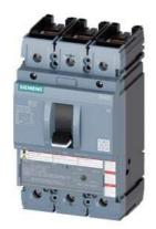
circuit breaker 3VA5 UL frame 250 breaking capacity class C 100kA @ 480 V 3-pole, line protection TM230, FTAM, In=150A overload protection Ir=150A fixed short-circuit protection Ii=5...10 x In UL489 SB (naval), 50 deg. cel. cable connection on both sides
