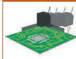
Inspecting Board Heights
