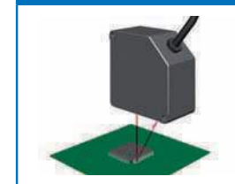
Inspecting for Board Coplanarity
