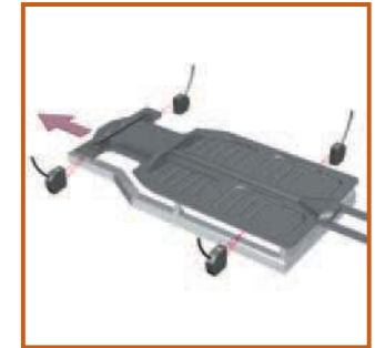
Measuring Car Body Widths (ZS-HLDS10)
