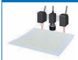
Inspecting Glass Heights (Autofocus)
