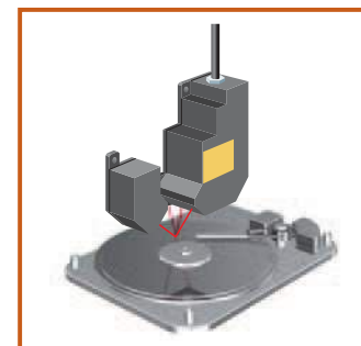
Inspection of Disk Play on HDD Motor Rotating Plate
