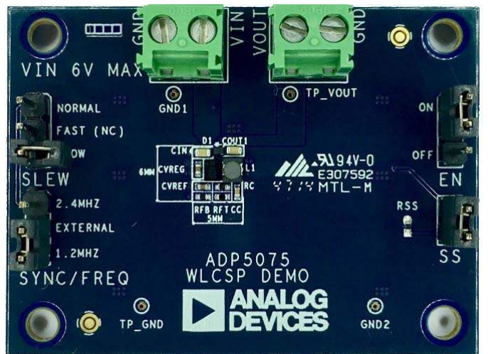
Figure 1. ADP5075CB-EVALZ Evaluation Board
