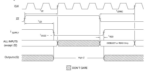
Notes: 20. Device must be deselected when entering ZZ mode. See truth table for all possible signal conditions to deselect the device. 21. DQs are in high-Z when exiting ZZ sleep mode.
